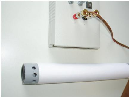
music on the speaker, we can hear thinner sound. The high pressure in front of the membrane and the low pressure behind it will generate acoustic wind; the waves will find the shortest path through the holes. In order to make its way longer, we can cover the holes by a paper roll, and the perceived sound becomes immediately much richer.
